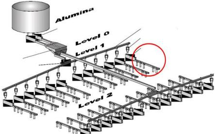
Figure 1. Example of Aerated Distribution System.
